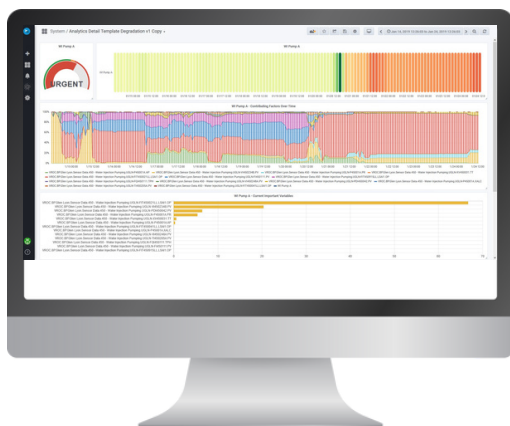
Dashboard showing Urgent Status for a system, with contributing factors for the predicted deviation.
