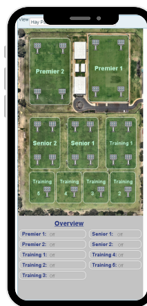
Mobile view of interface to control sporting field lights
